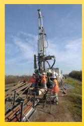
Geotechnical field crews drill borings to collect soil samples from a flood control levee.
