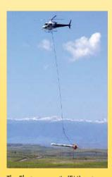
The Electromagnetic (EM) system collects three-dimensional earth resistivity data via a transmitter and receiver housed in the cylindrical "bird" slung beneath the helicopter.
